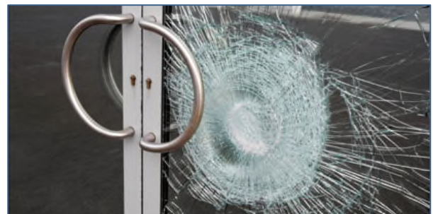
Fractured Glass in Door Protected by Security Window Film
